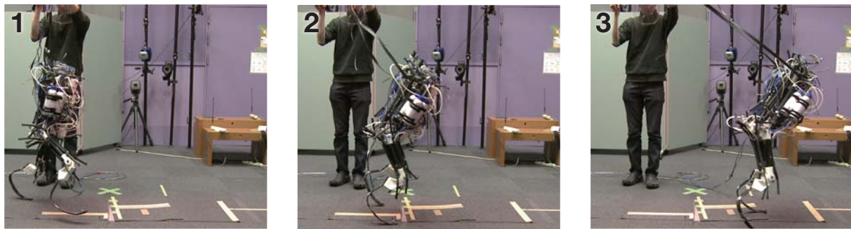
Fig.9 Snapshots of the three steps of bipedal running.
