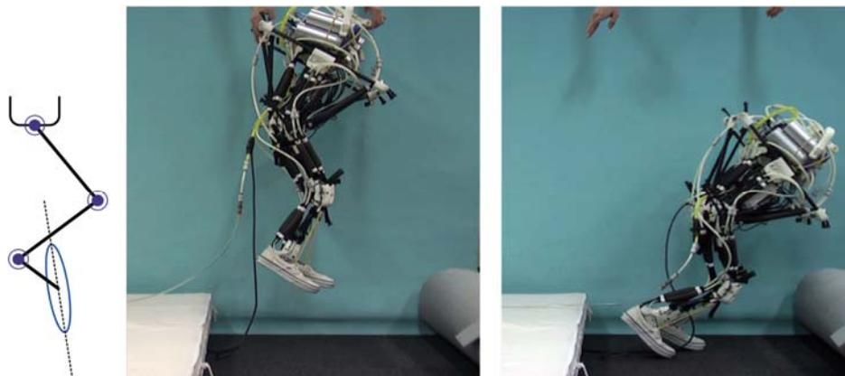
Figure 12 Passive control of bouncing by the preset stiffness (fall backward).
