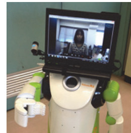
Figure 4: Teacher's view of the child operator on a Skype monitor mounted on the neck of the robot.
