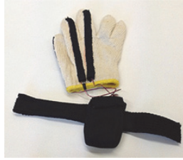
Figure 1: Data glove equipped with bending sensors extending along the fingers and a motion sensor that was attached on the wrist together with a Bluetooth circuit.
