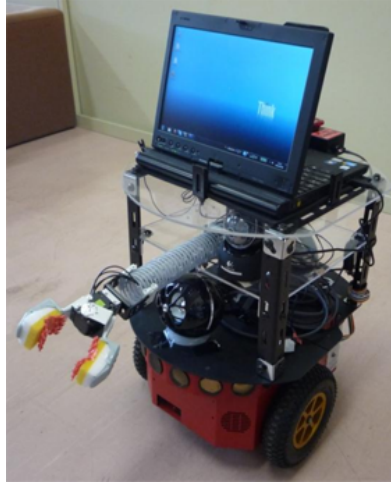
Figure 4: A telepresence robot remotely controlled by children. The operator’s face is projected onto the laptop LCD screen using Skype. The robot is built on a Pioneer P3-DX mobile robot base and equipped with a 1-DOF gripper hand, both of which can be remotely controlled using either the tricycle-style operation interface (Figure 2) or the video-game controller (Figure 3).
