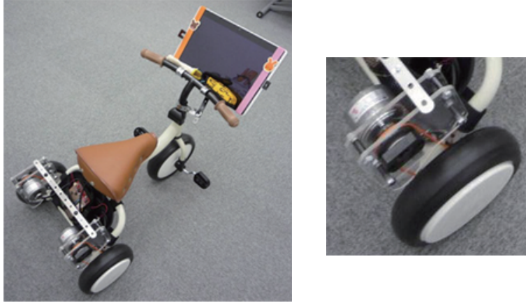
Figure 2: Second prototype of the tricycle-style operation interface. The 3-axis accelerometer of Figure 1 is replaced by two rotary encoders affixed to the rear wheels of the tricycle. The encoders detect more precise movement of the tricycle base.
