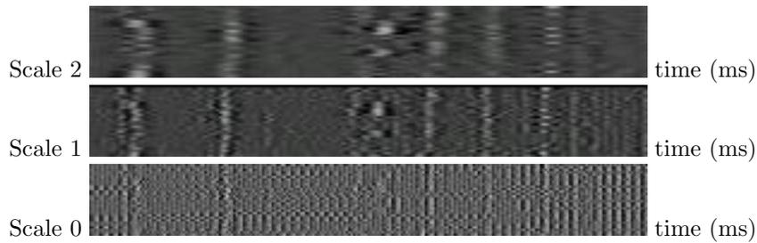
Fig. 1.6 Wavelet bifurcation diagram at different scales. In all three scale-plots, the horizontal axis denotes time (0-500 msec), and the vertical axis is the index of the chaotic unit.
