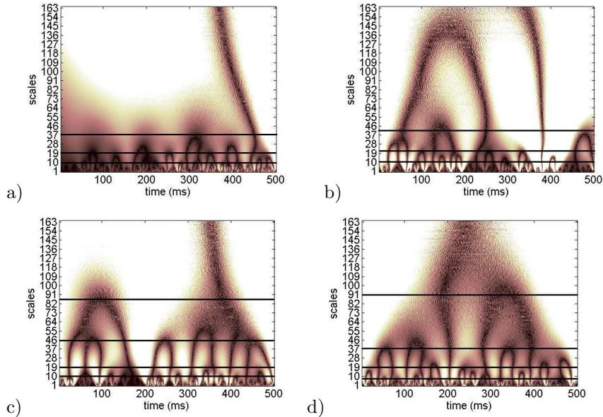
Fig. 1.5 Wavelet Transform. The spectro-temporal correlations between chaotic units are displayed. The control parameter  $\alpha$  varies linearly in the time interval 0-500 msec from (a) [0.0;0.5], (b) [0.5;1.0], (c) [1.0;1.5] and (d) [1.5;2.0].
