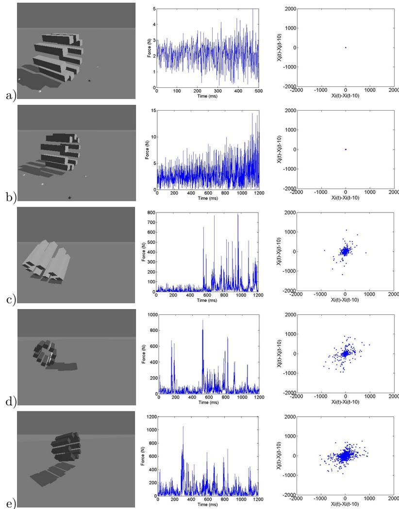
Fig. 1.3 Left: Snapshots of different postures for different  $\alpha$ ; (a) balance ( $\alpha = 0.05$ ), (b) rolling ( $\alpha = 0.10$ ), (c and d) quick and unstable movement ( $\alpha = 1.0$  and  $\alpha = 1.5$ ), and (e) uncoordinated movement pattern ( $\alpha = 1.9$ ). Center: Time series of one joint force pressure (unit: N). Right: Time-delayed phase portraits of two arbitrarily selected neighboring joints as a function of  $\alpha$ .
