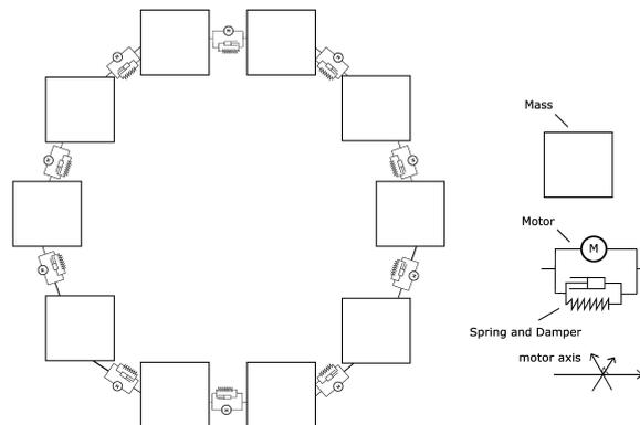
Fig. 1.2 Schematic representation of our robot model. The masses are prisms and are connected to each other by force-controlled compliant linear actuators. The system has 30 degrees of freedom.
