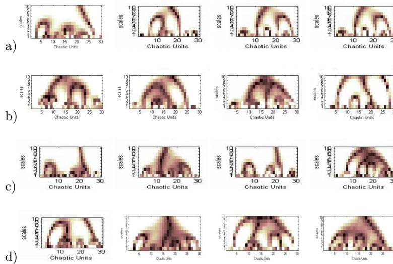
Fig. 1.7 Wavelet bifurcation diagram at different time instants. Snapshots of different neural configurations taken at different time instants for varying levels of chaoticity: a)  $\alpha = 0.5$ , b)  $\alpha = 1.0$ , c)  $\alpha = 1.5$ , d)  $\alpha = 1.9$ . The horizontal axis denotes the index of the chaotic unit, the vertical one is the scale (adimensional).
