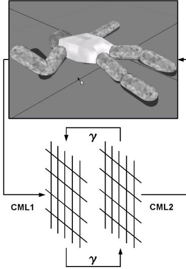
Figure 4: Outline of our embodied model system. "Body-CML 1" and "CML2-body" form two self-sustained oscillators.
