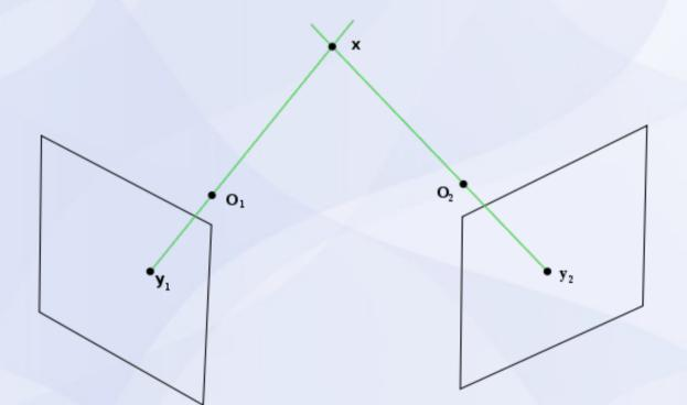
Corresponding image points are the projection of a common 3D point
