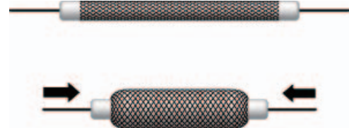
Fig. 8. Diagram of pneumatic muscle
