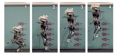
Figure 10 Soft landing from drop off height of 1.0 meter.
