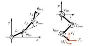
musculoskeletal legs with various muscle configurations as the pilot study. The joint angle, joint torque and output force at the contact point are defined as follows.
