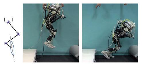
Figure 12 Passive control of bouncing by the preset stiffness (fall backward).
