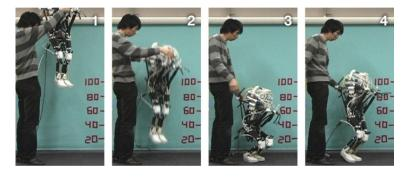
Figure 11 Passive control of bouncing by the preset stiffness (fall forward).
