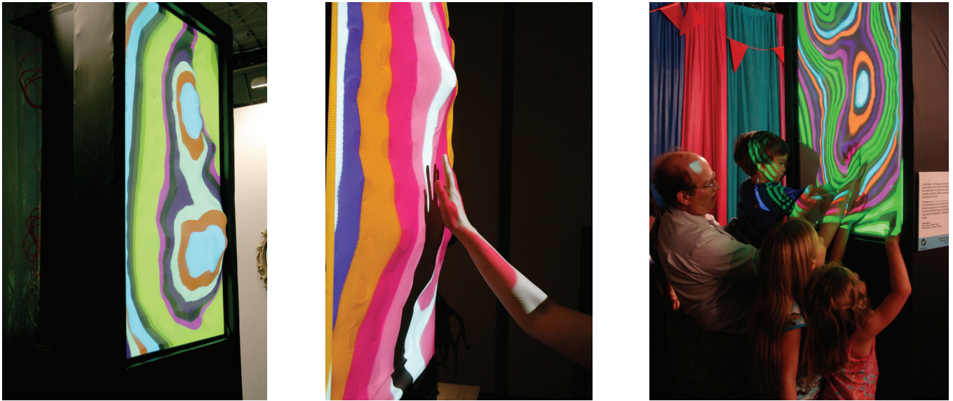
Figure 11: Demonstration of the prototype “Gemotional Bumpy Screen” at SIGGRAPH 2006 Art Gallery. The size of the screen was 0.6m×1.0 m (width × height). The actuator array was 6×12 (= 72 points), with an interval of 0.075m between points.
